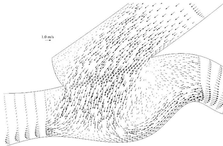
**Figure 5.** Velocity vectors at the symmetry plane of the junction region.
