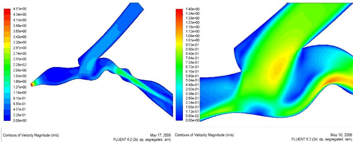
**Figure 4.** Velocity magnitude at the symmetry plane (left) and zoom in on the junction region (right).
