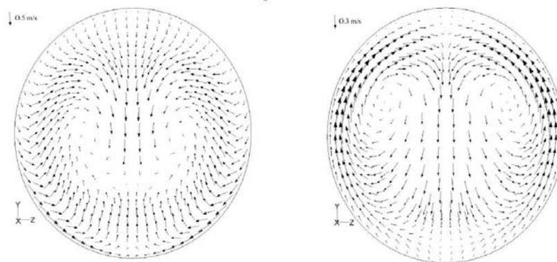
**Figure 7.** Velocity vector plots showing Dean vortices at cross-sections of the junction region. Proximal segment (left); distal segment (right).
