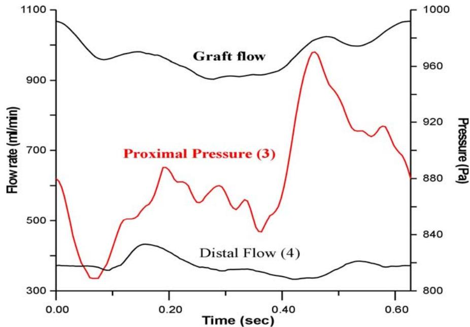
**Figure 2.** Recordings of flow rate at the graft inlet (black line) of pressure (red line) at the distal outlet (position 3) and of flow rate (black line) at the proximal outlet (position 4).
