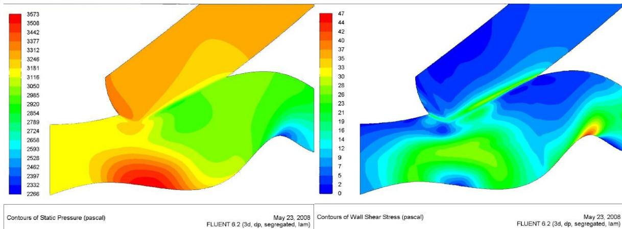
**Figure 6.** Contours of wall static pressure (left) and wall shear stresses (right) at the junction region.
